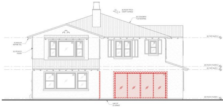
EXISTING / DEMOLITION WEST ELEVATION (REAR) NTS
